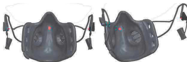
Figure 4 Different visual angles of the mask internal surface (the positions of the sensors are highlighted in red).
