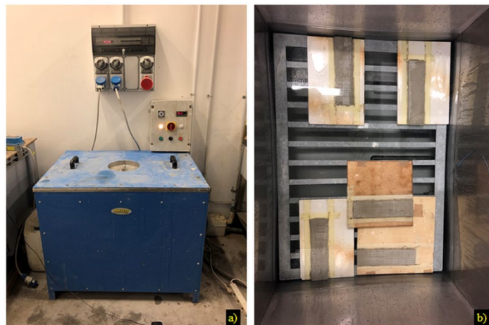
Figure 3. Curing conditions: a) accelerated concrete curing tank; b) 5 FRIL-panels immersed in water.
