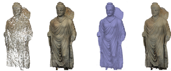
Figure 9. Sparse, dense cloud, mesh model, textured model.
