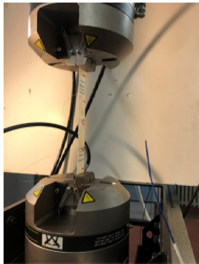
Fig. 5. Tensile test of specimens equipped with optic fibre.
