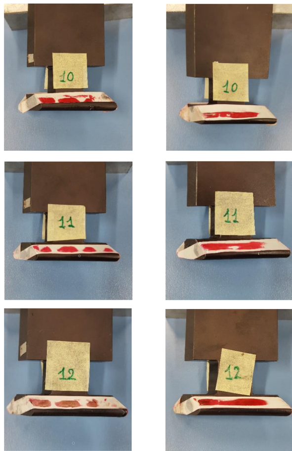
Fig. 6.1 Testing the static contact conditions on three different blades on the VITAL bladed-disk. The left and right pictures of each blade correspond to the two contacting sides [187].
