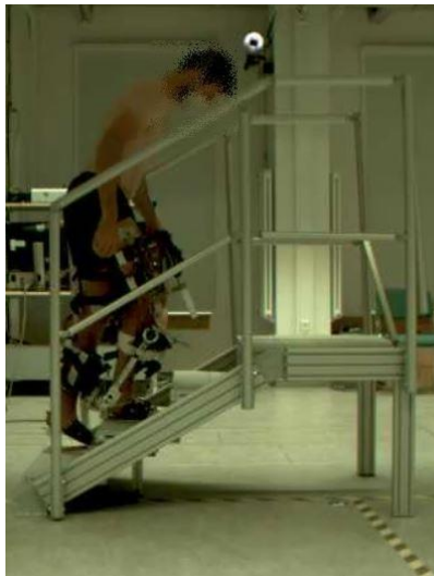
Figure 13: Trial of a stair ascent with the supporting exoskeleton on both legs. The experiment was conducted at the biomechanical lab of the University of Leipzig.
