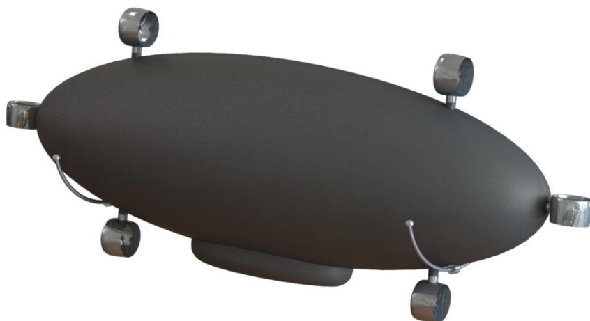
Figure 1 – Qualitative 3D rendering of the airship during flight (with the landing gear rotated inward).
