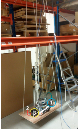
Fig. 4. Pitch/roll estimation testbench
