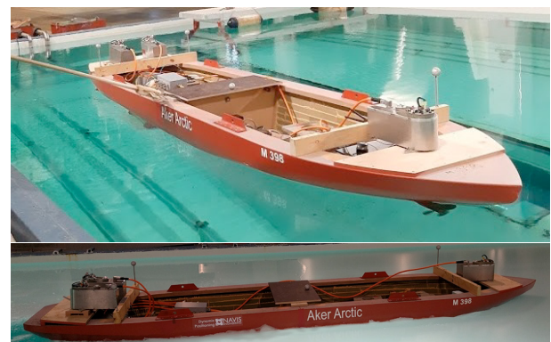
Fig. 12. Towing tank tests with Aker Arctic (Polaris icebreaker model), January 2019
