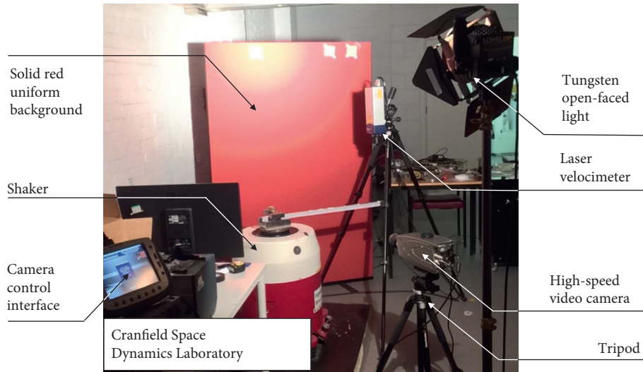
FIGURE 3: The second experimental setup (cantilevered box beam, Cranfield University).
