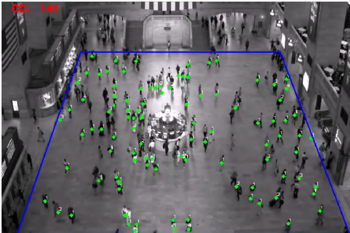
Figure 2.10: 'crowd counting people' (studied by Loy et al. in [174], Ryan et al. in [237] and Chan et al. in [63]). This methodology differs from the 'optical flow analysis' because the exploited camera focuses on the area to be analyzed while a software counts the people in the framed area.
