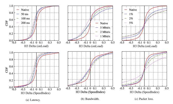
Fig. 7: H3 Delta on different scenarios. onLoad (top) and SpeedIndex (bottom). Negative values indicate that HTTP/3 is faster.
