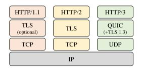
Fig. 1: Protocol stack for different HTTP versions.
