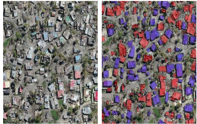
Figure 1. On the left: Orthophoto of Beira in 2019 after the cyclone Idai. On the right: WFP's DEEP software shows damaged houses in red and undamaged ones in purple — patchwork drone imagery turned into a detailed map. Image: WFP.
