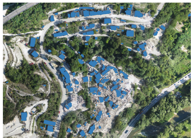
Figure 3. Automatic building segmentation performed by Deep on the Pescara del Tronto 2016 orthophoto. The recognized building footprints are represented in blue color.
