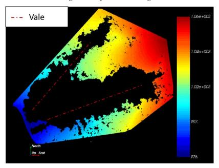
Figure 5 - Spatial distribution of terrain elevation data, with the notable absence of data in the valleys, where the vegetation is dense.
