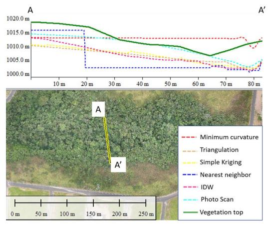
Figure 7 - Cross-sectional profile of surfaces generated by conventional interpolators.
