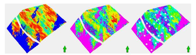
Figure 1 – Synthetic 'truth'. Left to right, NTG, NET and PORO for a representative layer in the model. The locations of the well samples are superimposed on the PORO image.
