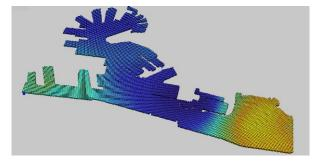
Figure 1 – Geometric model with structured grid (voxels of equal size) where the distribution of a synthetic variable is simulated.
