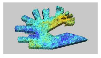
Figure 5 – Geometric model with unstructured grid (tetrahedra) where a synthetic variable is simulated.
