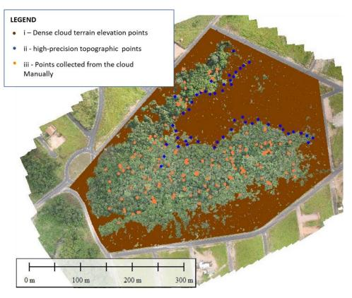
Figure 6 - Types of terrain points according to the acquisition method.
