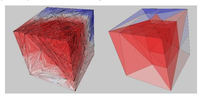
Figure 2 – Cubic geometric model with unstructured grid (tetrahedra) of a cube 100x100x100 meters. On the left: the synthetic reality on the fine-scale unstructured grid; on the right: the averaged synthetic reality on the coarse-scale unstructured grid
