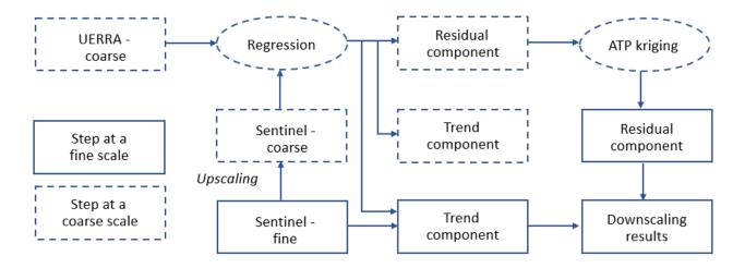
Figure 3: Flowchart of ATP Regression Kriging (ATPKED) Spatial Downscaling Algorithm
