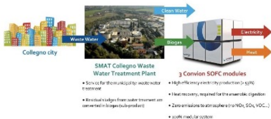
Figure 3.1. Waste-to-Energy production system at SMAT's WWTP (DEMOSOFC)
