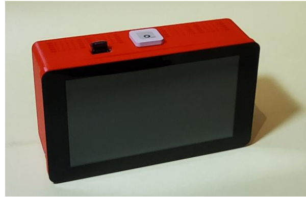
Figure 10: Handheld device and touch screen for the direct Space-to-ground decryption and visualization (used for the S-band data link transfers)
