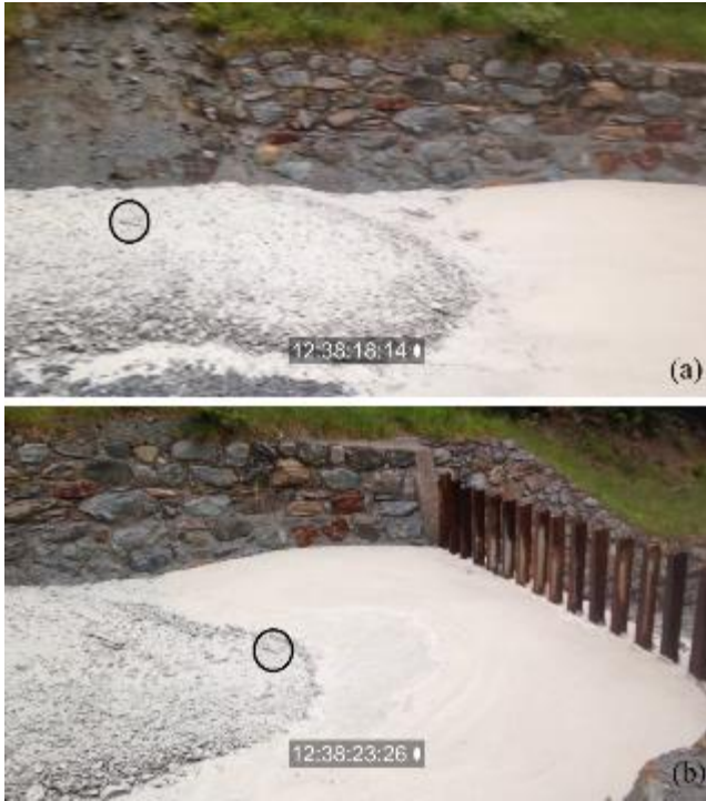
Fig. 8 Event on 9 June: Example of particle-motion tracking as the video advances frame-by-frame. Note that before hitting the barrier, the front submerges into a pool of water accumulated behind the barrier, becoming undetectable. Therefore, we use the last available frames with a visible front for the particle tracking procedure.
