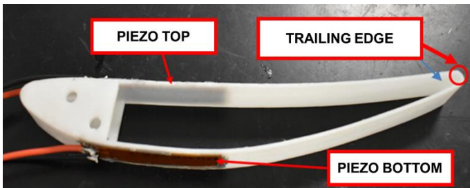
Figure 8 - Piezo positioning and TRAILING EDGE location
