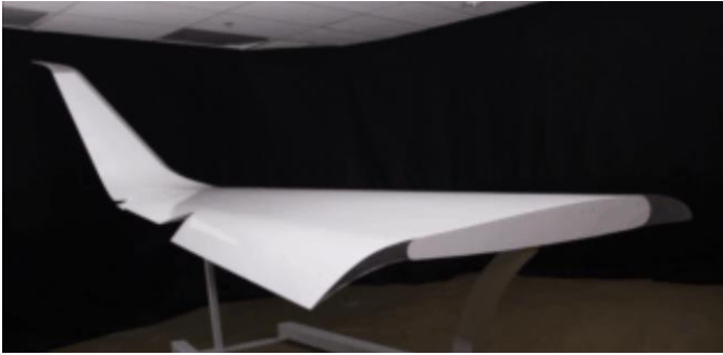
Figure 3 - Skin deformation of FlexFoil wing
