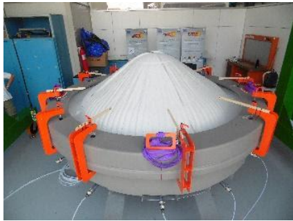
Fig. 19. HIAD demonstrator under static load testing.
