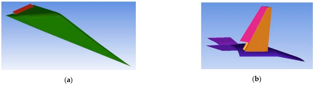
Figure 11. Simplified configuration of the Wing-Flap (a) and Body-Flap (b).
