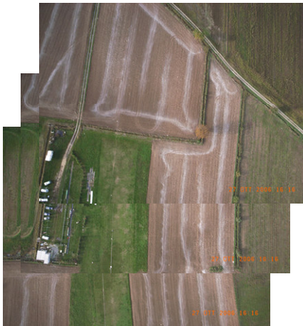
Figure 13. Frames used for the aerial triangulation
