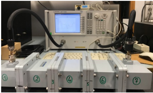
Fig. 3: Experimental set-up of the wave-guide technique.
