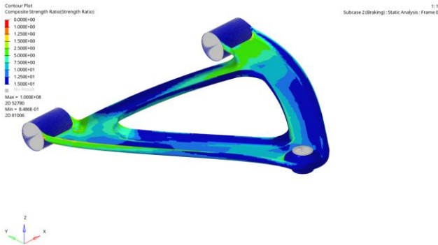
Figure 33. Contour plot of composite strength ratio: braking load case (shuffle optimization)
