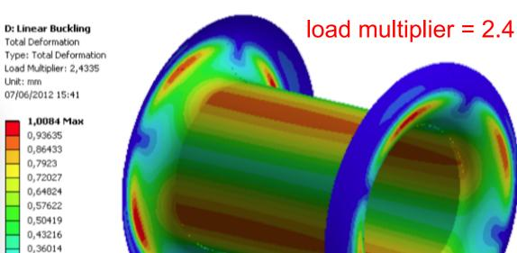
Inner cylinder sandwich: 2 C-fiber skins, 2-ply each, HM M30S 53 ET443 51% + C-foam core, 5 mm total **Grafoam® FPA-10** 0.100 g/cm<sup>2</sup> total
