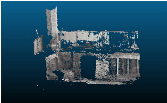
Figure 8. Sparse point cloud obtained with the manual selection of feature points workflow.
