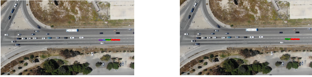
Fig. 8: Real-world dataset: Trajectory prediction when the vehicle approaches a standstill state without (left) and with (right) TLS information. Past observations (red), actual trajectory (green), predicted trajectory at t + 1 (yellow), t + 2 (blue), and t + 3 (purple).
