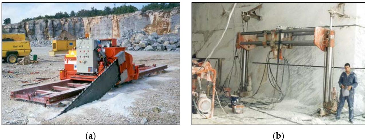
Figure 7. (a) A chain cutter operating on a bench to perform a vertical cut; (b) the version commonly adopted for underground use: the versatility of this machine allows the creation of additional free surfaces in bottom-blinded openings of “weak” stone quarries, for which it is very frequently adopted.
