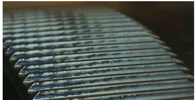
Figure 5. Effect of the coning angle on the flexspline tooth wear.
