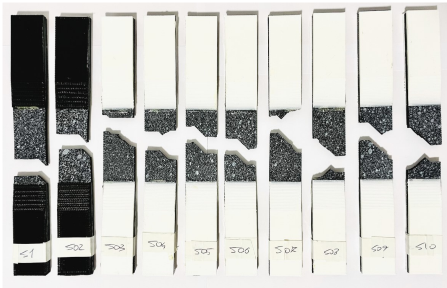
Figure 3.44: Specimens for shear properties determination at the end of the tests.
