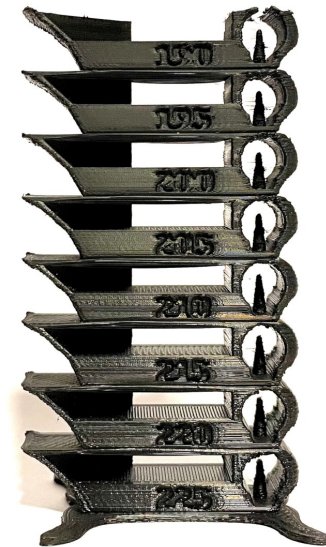
Figure 1.12: Temperature test for extrusion temperature quantification.
