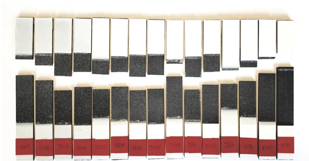
Figure 3.27: First DoE, tensile specimens loaded in direction 2 after the test.
