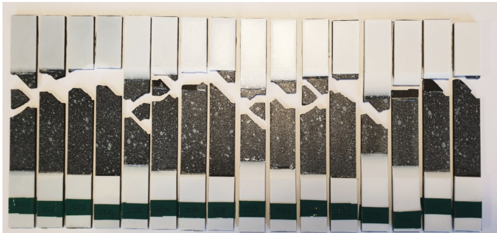
Figure 3.41: Second DoE, \pm 45^\circ shear specimens after the tests.
