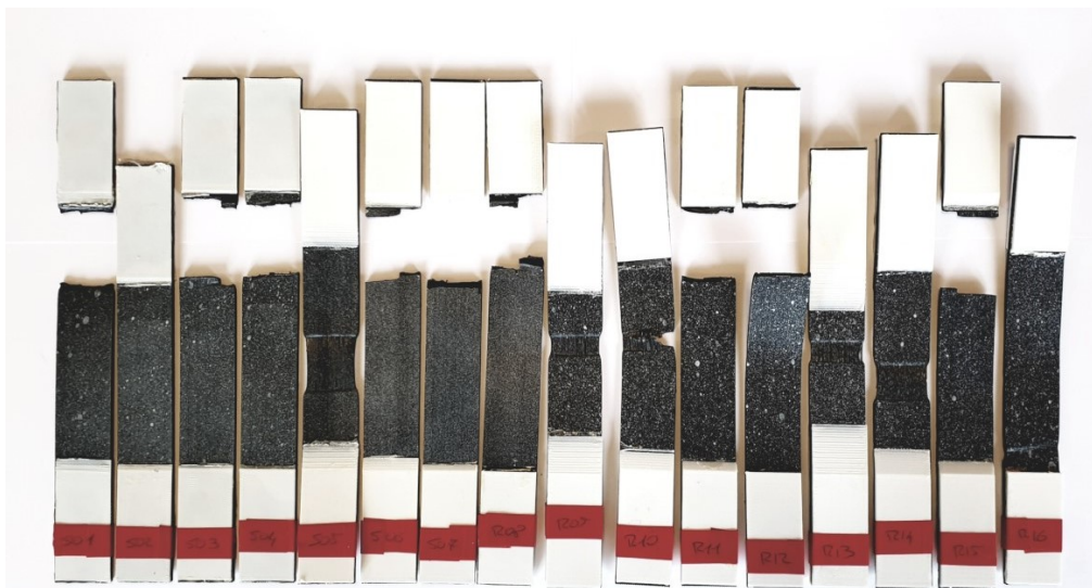
Figure 3.24: Second DoE, tensile specimens loaded in direction 1 after the test.
