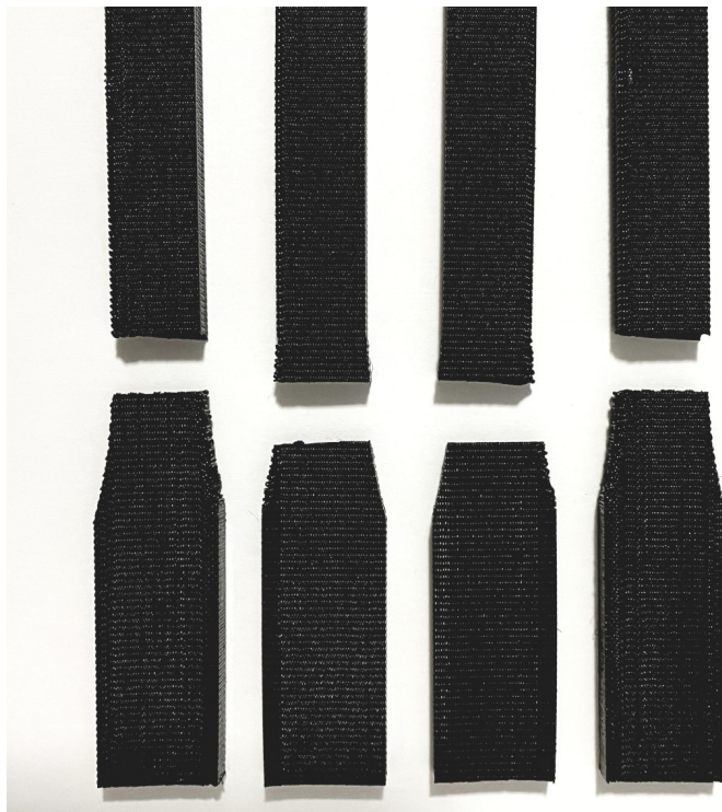
Figure 3.17: Failed dog-bone specimens for mechanical properties evaluation in direction 2 after the preliminary tests.
