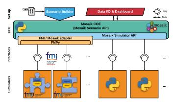
Fig. 1. Scheme of the distributed co-simulation infrastructure. It reports the enabling technologies and main elements of the platform: Scenario Builder, Data I/O & Dashboard interface, *Mosaik* COE including Scenario and Simulator APIs, FMI/Mosaik adapter, simulation blocks and their interfaces.
