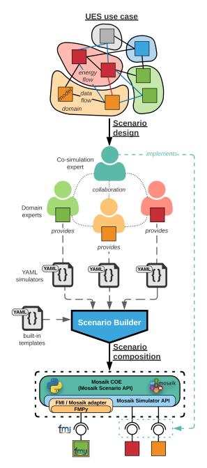
Fig. 2. Overview of the main steps to perform scenario design and composition starting from a UES use case within the co-simulation platform.
