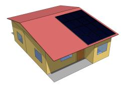
Fig. 5. The 3D layout of the house modelled with the OpenStudio suite and SketchUp plug-in.
