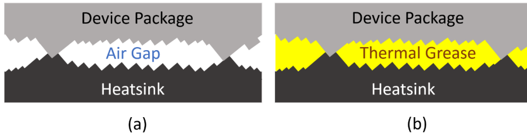
Figure 12 Heatsink-device mechanical coupling
