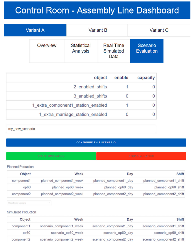
Fig. 6. User interface to configure a new scenario and its simulated throughput visualization.
