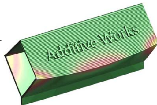
Figure 4. Geometry of the as-built AW Box with mesh structure for SLM simulation.
