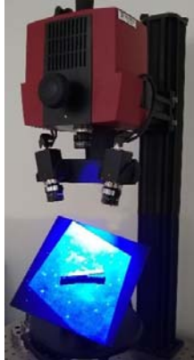
Figure 5. Inspection of a cantilever using the Atos Compact Scan 2M.
