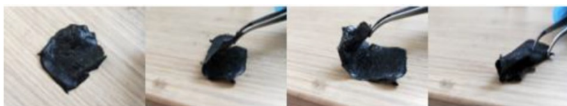
Figure 3.19: Cyclic bending and twisting to check the resistance to damage of the printed film.
