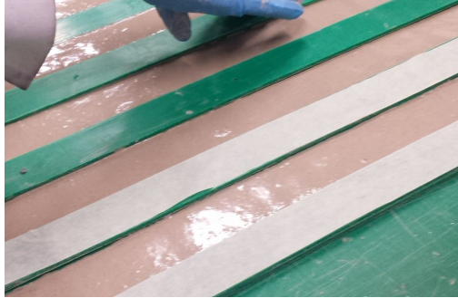
Figure 2: Manufacturing process of the specimens: application of the second set of constraining laths for uniform placement of the second layer of mortar
