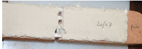
Figure 7: Typical telescopic failure mode for brick bending in the G-UC specimen group
