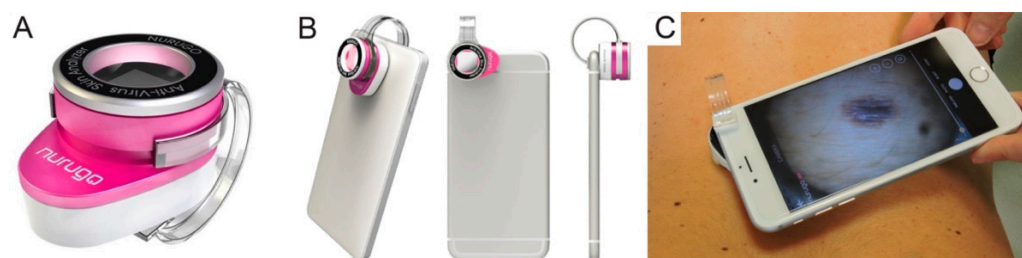
Figure 2. (A) Nurugo TM Derma; (B) Nurugo TM Derma attached to the smartphone; (C) Example of smartphone microscope applied to skin.
