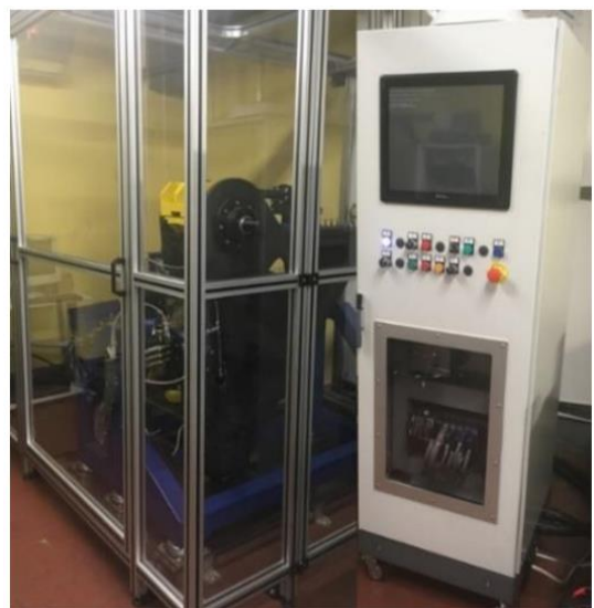
Fig. 5. Test bench for PHM on EMA flight controls [2]
