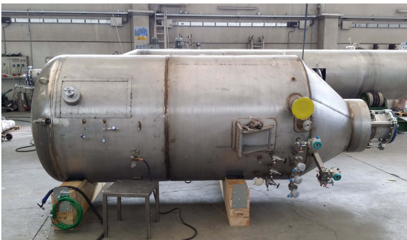
Fig. 4 The bottom module of the column.
