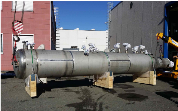
Fig. 3 The top module of the column.
