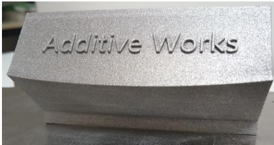
Figure 5. Ti6Al4V replica of the reference square tube by Additive Works.
