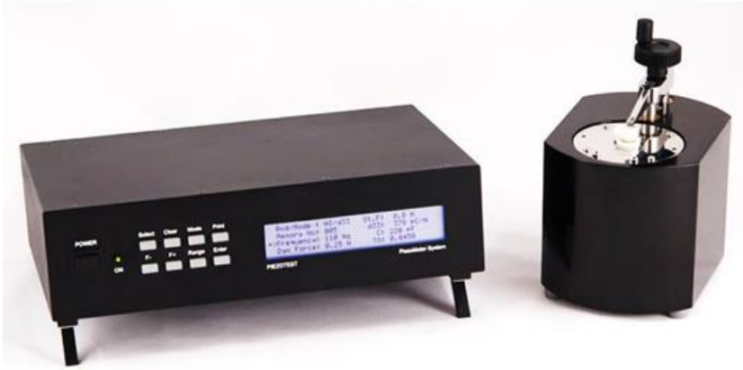
Figure 2.5. Piezotest PM200 employed for the calculation of d_{33} values of the analyzed samples.
