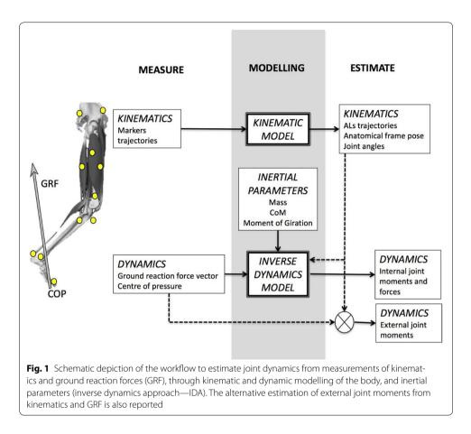
The first is the so-called inverse dynamics approach (IDA): the human body is represented as a multi-body chain of rigid segments, and Newton–Euler mechanics is applied iteratively to each segment to calculate net internal joint moments and forces [1–4]. *Marker trajectories* from stereophotogrammetry and *ground reaction forces* (GRF) from dynamometric platforms ("force platform" in short), are the input to the *kinematic* and *dynamic models* of the human body.
