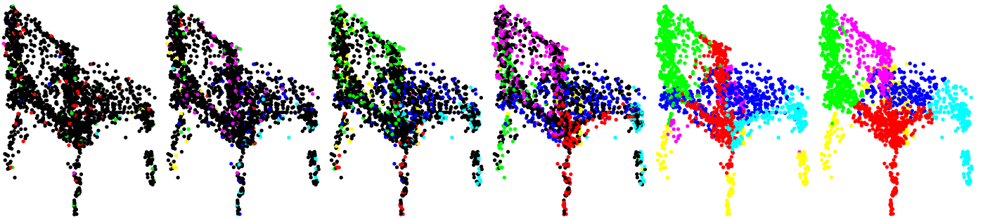
Fig. 11: Probabilistic upsampling: k -means clustering of features of intermediate layers after upsampling, highlighted onto the output point cloud (leftmost: output of dense layer, rightmost: output point cloud). Black points are not yet generated at the intermediate layers. Notice how the generated points are almost uniformly distributed and how the layer features create neighborhoods that are progressively more localized with respect to the output geometry.
