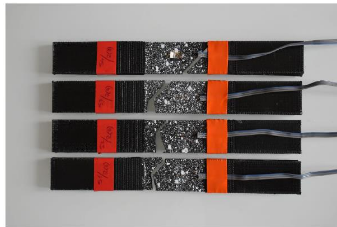
Fig. 7: Run(B) specimens after the tensile test ended
