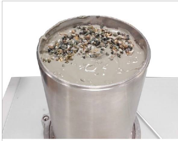
Figure 7.4: Blocks added in half of the consolidometer cylinder to obtain 50%VBP specimens.
