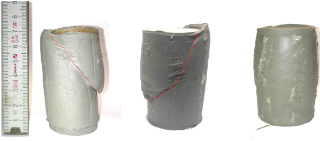
Figure 7.8: Failure modes of the three homogeneous specimens tested. From the left: specimens 1 (localized failure), 2 (localized failure) and 3 (diffuse failure), after the tests.
