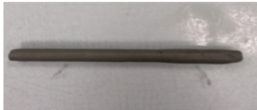
Figure 6.13: 3 mm diameter thread for the determination of the w_P of sample n.1
