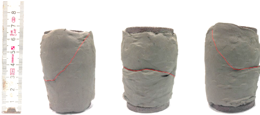
Figure 7.14: Failure modes of the heterogeneous specimen with 25% VBP.
