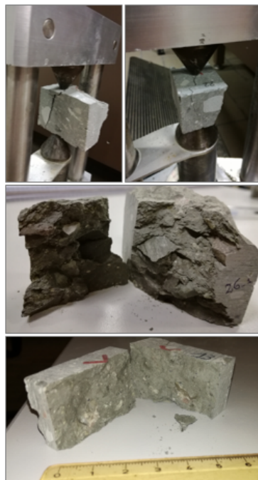
Figure 6.33: Typical samples successfully tested with the PL apparatus: the failure surfaces pass through both the platen loading points.
