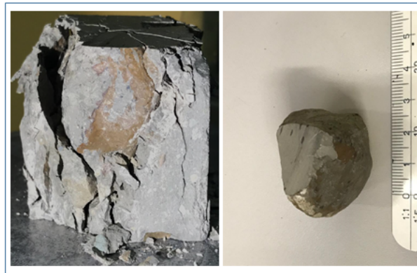
Figure 6.40: A 2 cm overconsolidated clay inclusion within a heterogeneous melange specimen failed in uniaxial compression. The result of this test was discarded because it was considered not to be representative.
