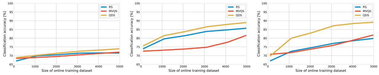
Fig. 4. Classification accuracy as a function of the size of the online training set, for different data selection strategies, under the labels (left), data (center), and samples (right) modes.
