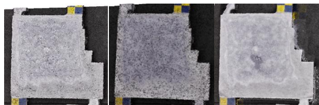
Figure 2. Examples of point cloud referred to nadiral (left), oblique (centre) and nadiral+oblique (right) images
