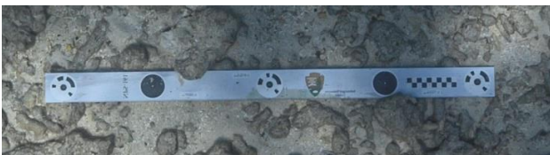
Figure 4. One of the three calibrated scalebar used for scaling the model.
