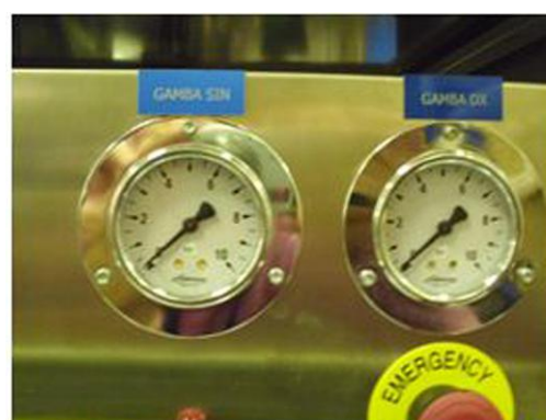
Figure 4: Pressure manometers in the fixed box used to set and to read the pressure in the two legs of P.I.G.R.O.
