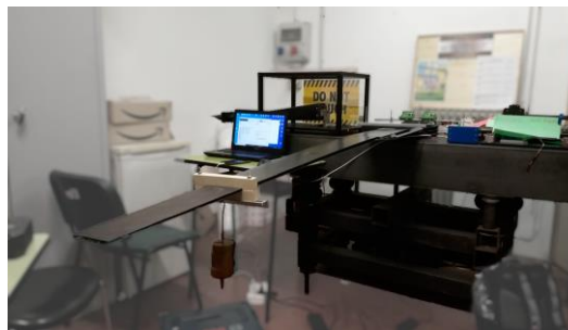
Fig. 7. Experimental setup for the static load tests on the wing
