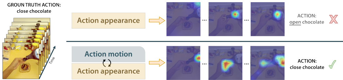
Fig. 1. By leveraging a self-supervised motion prediction task during training, at test time, SparNet can jointly exploit motion and appearance information using a single RGB stream. The result is a leaner architecture that better focuses on the relevant elements for action recognition in egocentric vision, as can be seen from the comparison between the Class Activation Maps when the auxiliary task is used (lower path) or not (upper path)
